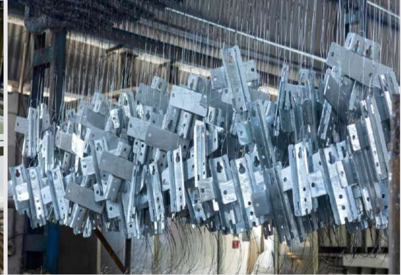
Hot Dip Zinc galvanization
